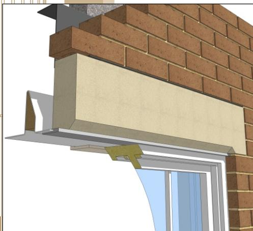
Our Heads are non structural and should be used in conjunction with supporting lintels.
