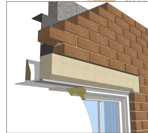
Typical installation detail
