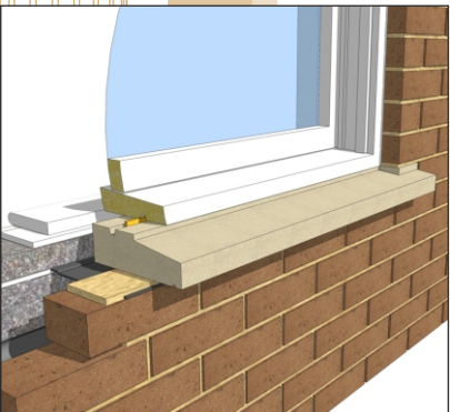
Typical installation detail
