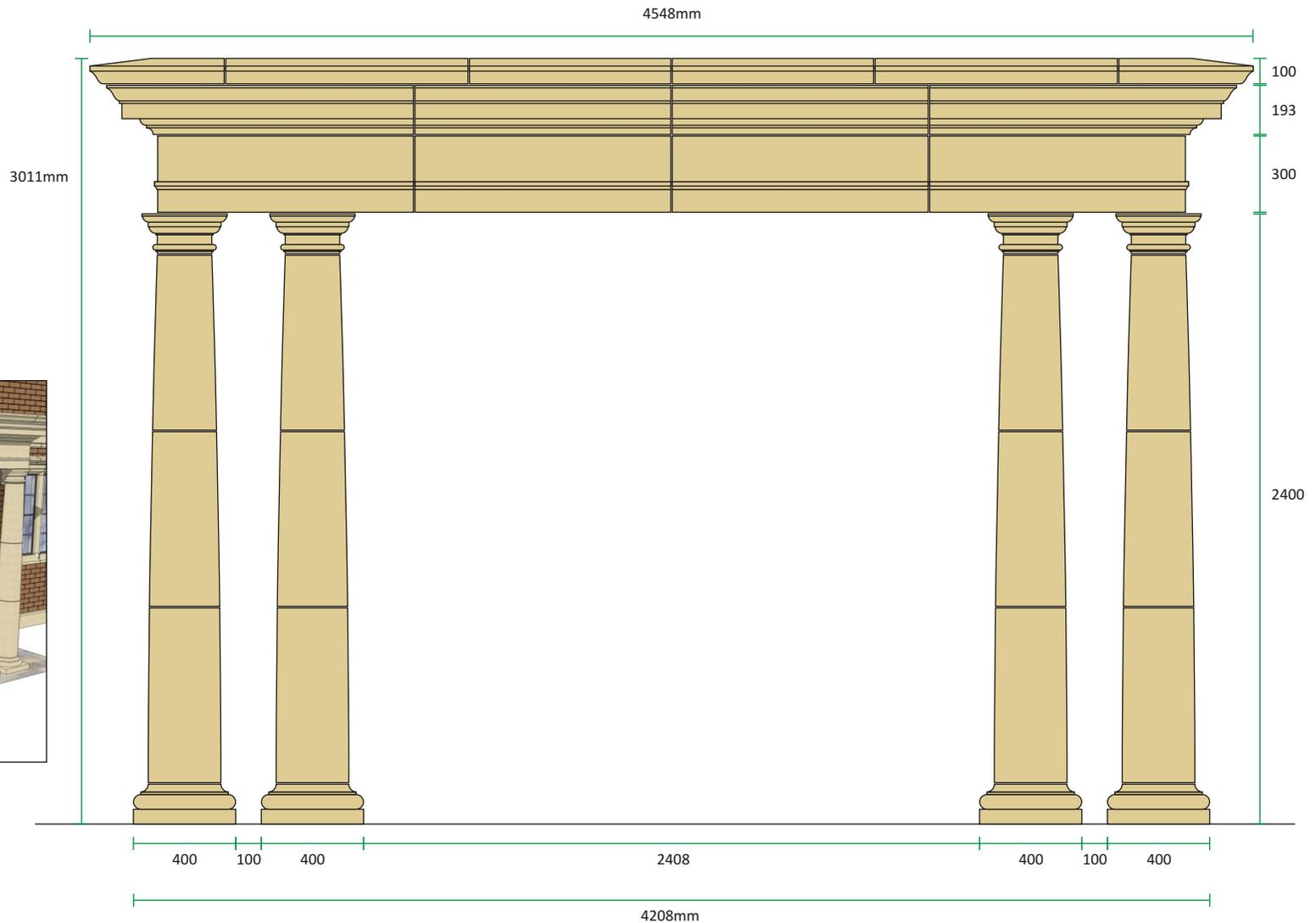
This example has a maximum projection from the building of 1531mm
